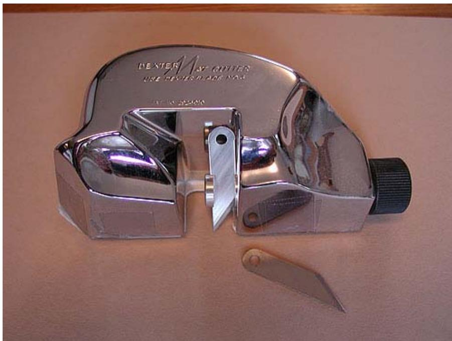
The Dexter is a hand held device which holds a blade positioned at a 45 degree angle so that your cut will be beveled. To cut simply measure and trace the opening as described above and use a straight edge ruler to guide the Dexter. Make sure that you over cut each side 1/4" approximately so that the opening will fall out after you are done cutting it. The over cut is necessary because the bevel makes the opening on the back of the mat slightly smaller than the opening on the front of the mat.
